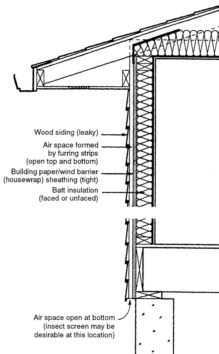
In summary, ventilating horizontal lap siding may improve its service life. If the siding is installed using a rain screen design, the rainwater will probably not penetrate past the siding. Installing horizontal lap siding using the rain screen method is also reasonably inexpensive and easy to execute.
