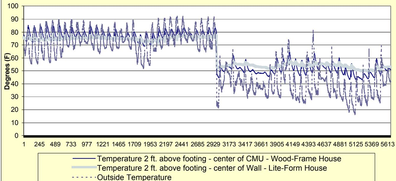
foundation/insulation/slab detail of the wood-frame home represents a significant source of heat loss and gain not evidenced in the ICF homes.
