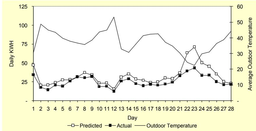
**Figure 19 – Wood frame Energy Consumption, Predicted vs. Actual (February 1999)**
