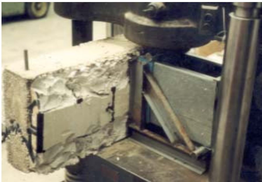
Figure 4 Photograph of Test Set-Up
