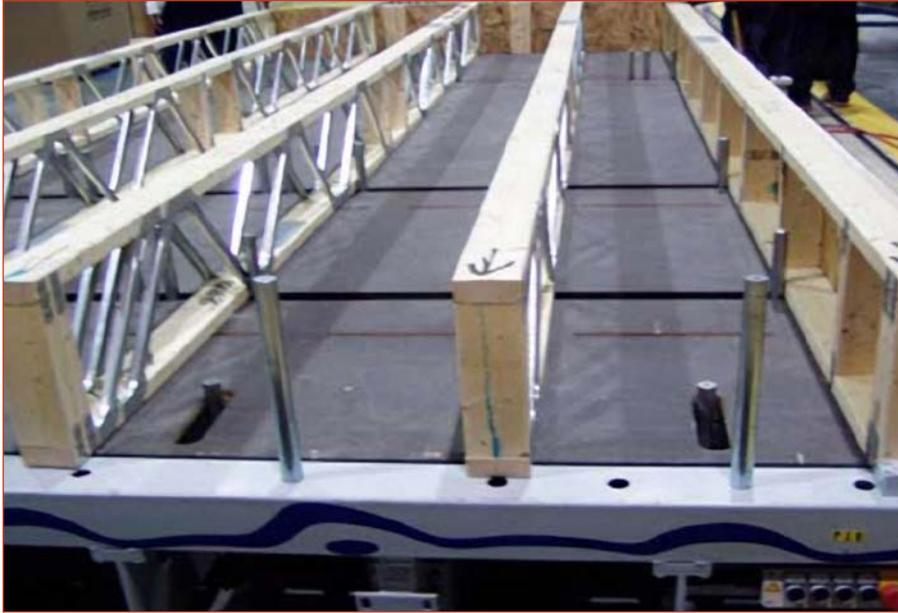
Open metal web floor trusses are precisely positioned by the floor deck assembly machine.
