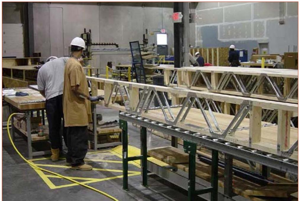
A quality operator performs a visual check and stages trusses immediately after automated assembly.
