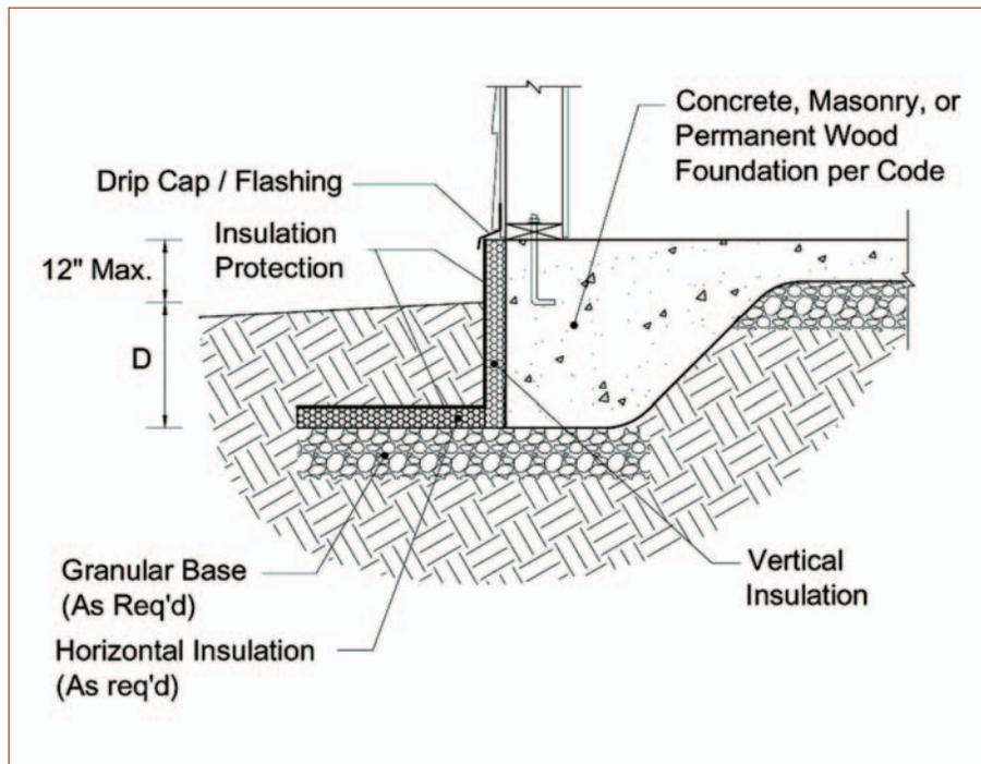
Figure 1. Section detail showing properly placed insulation protection.<sup>1</sup>
