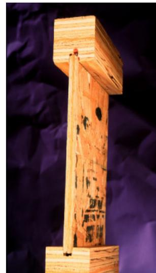
Wood I-joist with LVL flanges and OSB web material
