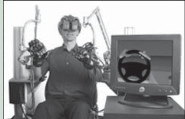
**Simulated automotive steering using the Haptic Workstation.**
