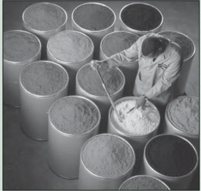
**Sampling drums of ARCTIC infrared-reflective powders.**
