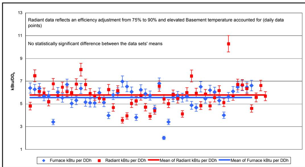
**Figure 6 Furnace and radiant system natural gas consumption per heating degree day (boiler efficiency to 90% and basement temperature differences accounted for) (daily data used)**
