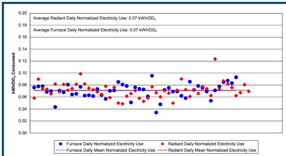
Figure 4 Furnace and radiant system electric consumption per heating degree day (daily data used)
