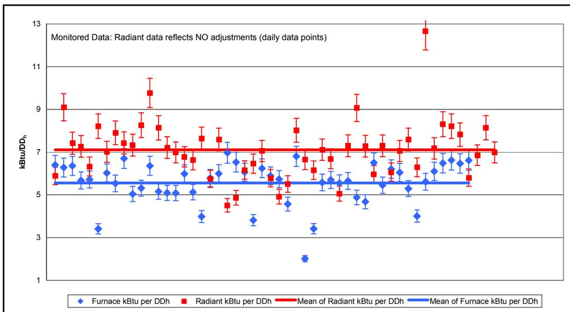
**Figure 5 Furnace and radiant system natural gas consumption per heating degree day (no adjustments to data) (daily data used)**
