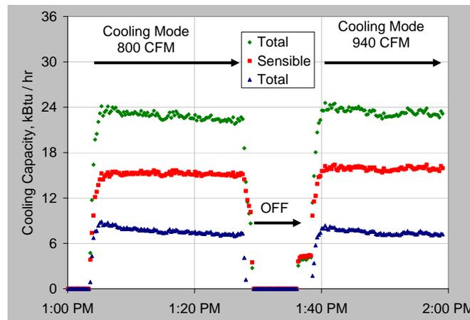
Figure 6. SEER 14 System Cooling Capacity on August 11, 2005
