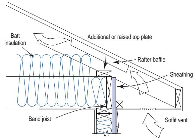
A raised top plate increases the height for insulation and ventilation at the eaves.
