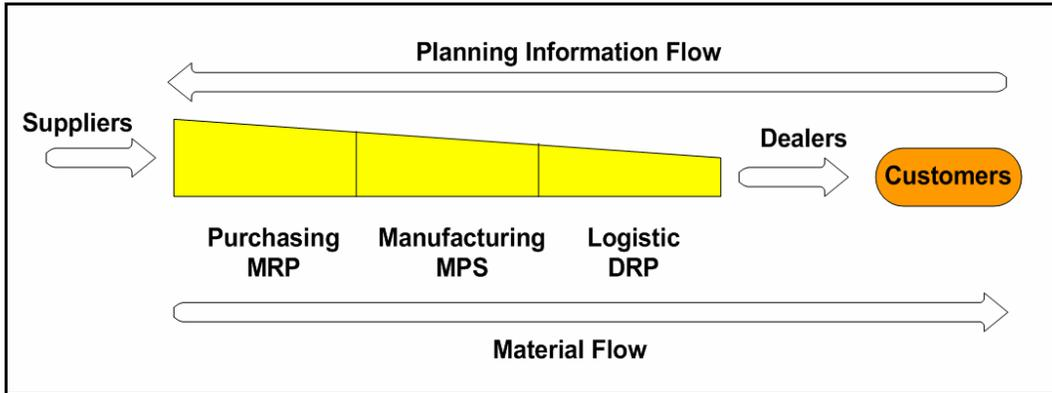
FIG. 2. Supply Chain Management System for Manufacturing Housing Industry (Barriga 2003)
