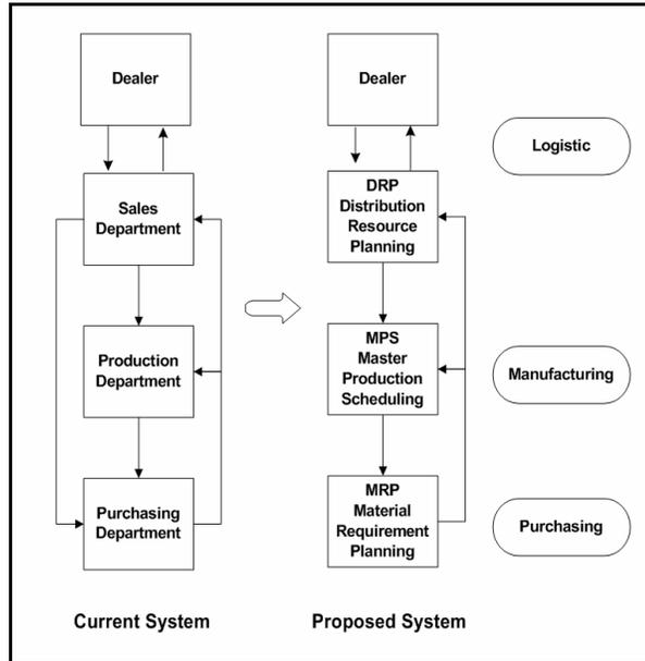
FIG. 3. Integrated Supply Chain Management System for Manufacturing Housing Industry
