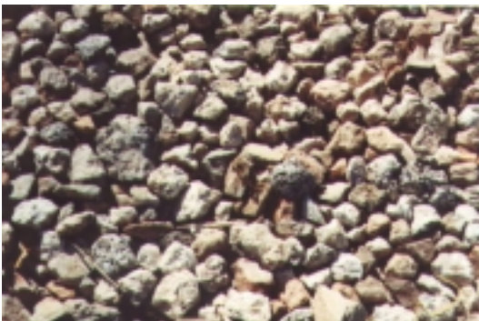
Recycled concrete backfill obtained from a local demolition site.
