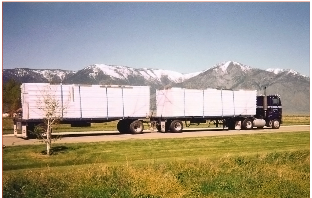
Most panel sizes are conducive for easy transportation. Panels are also labeled according to their placement to speed installation.
