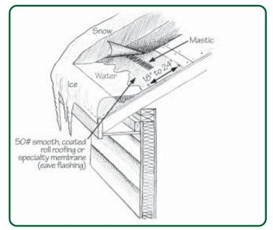
Figure 4.9 - Eave Flashing for Preventing Ice Dams
