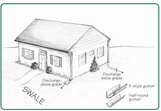
Figure 4.4 - Roof Gutters and Discharge Methods
