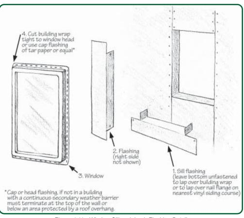
Figure 4.11 - Window Sill and Jamb Flashing Detail (building wrap installed after window)
