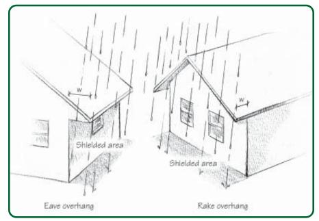
Figure 4.2 - Roof Overhangs
