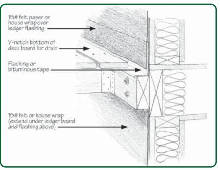
Figure 4.14 - Deck Ledger Flashing Detail
