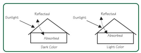
Figure 5.3 - Effect of Surface Coloration on Solar Heat Gain
