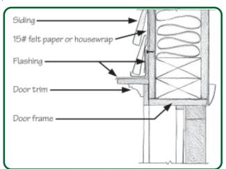
Figure 4.13 - Door and Head Trim Flashing Detail
