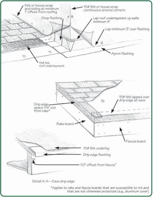
Figure 4.8a - Basic Roof Flashing Illustrations
