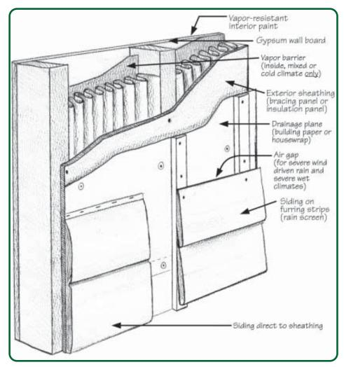
Figure 4.6 - Weather Barrier Construction
