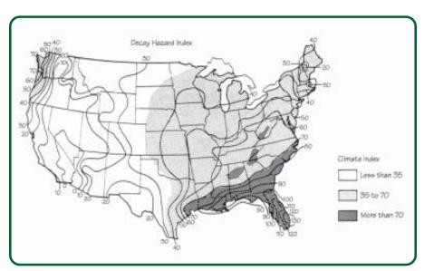
Figure 4.3 - Climate Index Map Based on Wood Decay Potential Prepared by the U.S. Weather Bureau.
