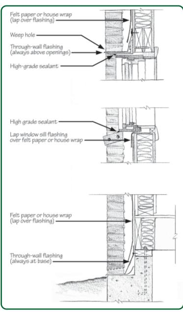
Figure 4.15 - Typical Brick Veneer Flashing Details
