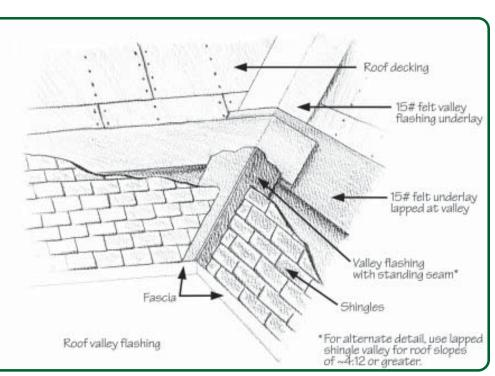
Figure 4.8b - Basic Roof Flashing Illustrations (continued)
