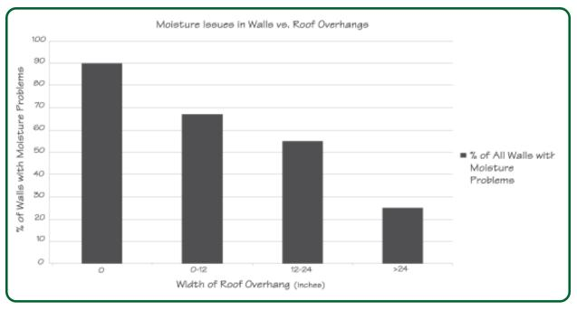
Figure 4.1 - Frequency of Moisture Problems in Walls of Selected Buildings in a Moist, Cool Climate (Climate Index of approximately 70 based on Figure 4.3)
