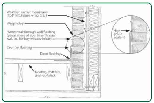
Figure 4.16 - Brick Veneer Flashing at Roof Intersections
